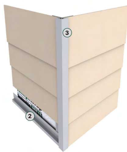
STARTER STRIP AT OUTSIDE CORNER
